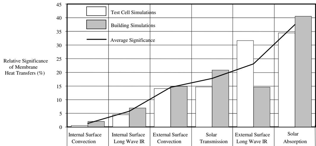
It can be seen that both of the predicted internal surface heat transfers were more significant for the buildings investigated than was the case with the test cell, whilst the significance of external surface long wave infra red radiation was considerably reduced. It was likely that this resulted from the fact that the test cell investigations could only be carried out during dry conditions, when there was likely to be little cloud cover.
