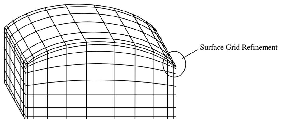
*Flovent* was unable to generate such a BFC grid. Some existing CFD codes are based on BFC grids (*Phoenixs*<sup>[27]</sup>) or even unstructured grids (*Fluent*<sup>[28]</sup>), but in order to accommodate some of the other developments suggested in this section, it seems likely that a purpose written thermal model may have to be developed.
