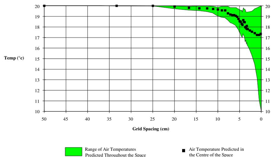
It can be seen that the predicted air temperature in the centre of the space decreased by almost  $2.75^{\circ}\text{C}$  as the grid spacing became smaller. This was as a result of *Flovent* being more able to simulate the fast moving down draft close to the cold surface, resulting in increased convection heat transfer at that surface.
