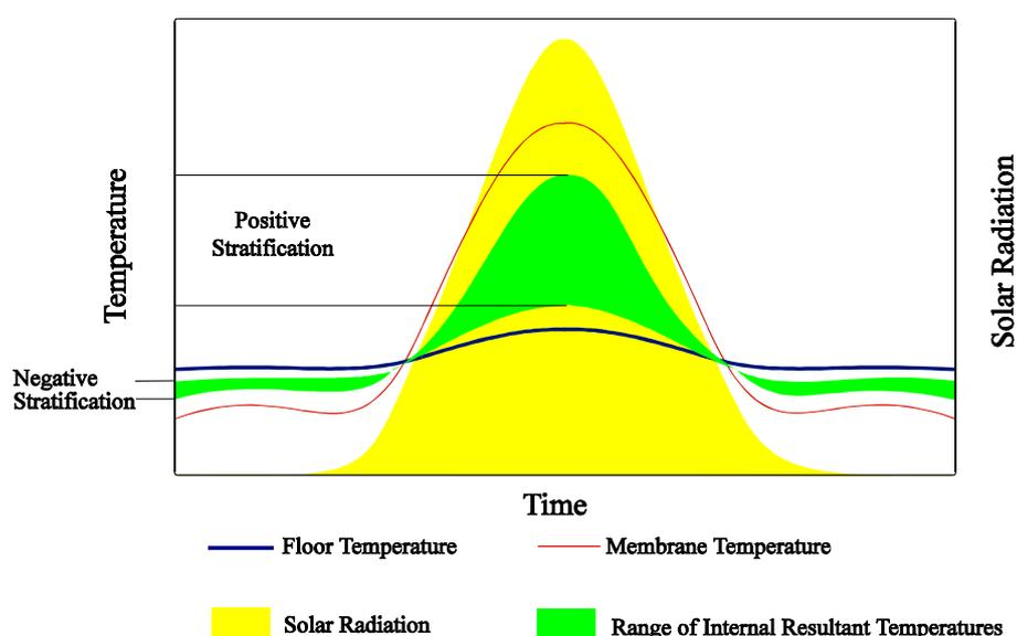
During periods of bright sunshine, fabric membranes were seen to heat up quickly and significantly, whilst at night or during cold clear weather, they could rapidly become considerably cooler than their surroundings. The contrast between this and the relatively stable thermal behaviour of more 'massive' internal surfaces such as the floor, meant that
