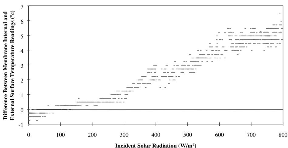
It seemed likely that the internal surface temperature reading was more representative of the temperature of the membrane than the external sensor as it was generally less exposed to severe external conditions. As this was also the surface which actually affected the behaviour of the enclosed space, it seemed reasonable that the research presented in the rest of this thesis should concentrate on these *internal surface temperature* readings.
